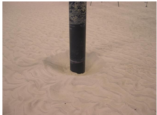
Example of scour around cylindrical pile, similar to that used for offshore windfarms.
